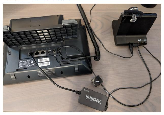
The box-of-matches-sized-device labeled EHS plugs into the EXT port on the phone, and the AUX port on the Headset. The cable with one phone cord end plugs into the headset port on the phone and it's other Ethernet-type end plugs into the physical headset base. It can get even more complicated than this if your phone also has a busy indicator light (shown at left) that lights to alert others whenever you are on the phone - this is useful because it is often not obvious to
